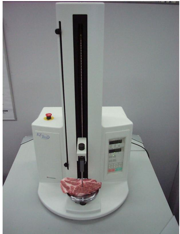
Fig. 2 Penetrating Strength Test Being Performed on Pork
