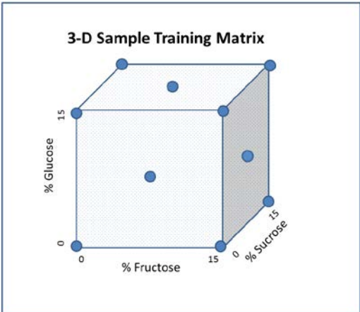
Figure 3: 3-Dimensional cube showing placement of training matrix calibration samples
