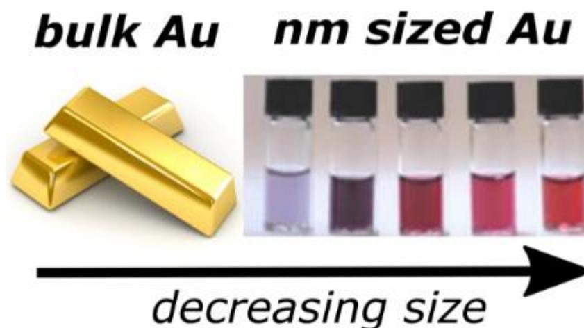
Figure 2: Change in the optical properties of gold as the size of its particles decreases.
