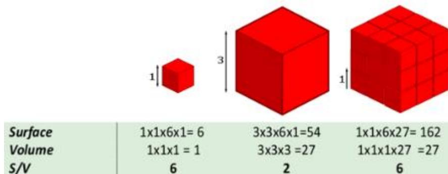
Figure 1: Increased surface to volume ratio for materials comprised of particles compared to bulk.
