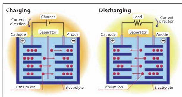
Fig. 1 Schematic of a Lithium Ion Battery
