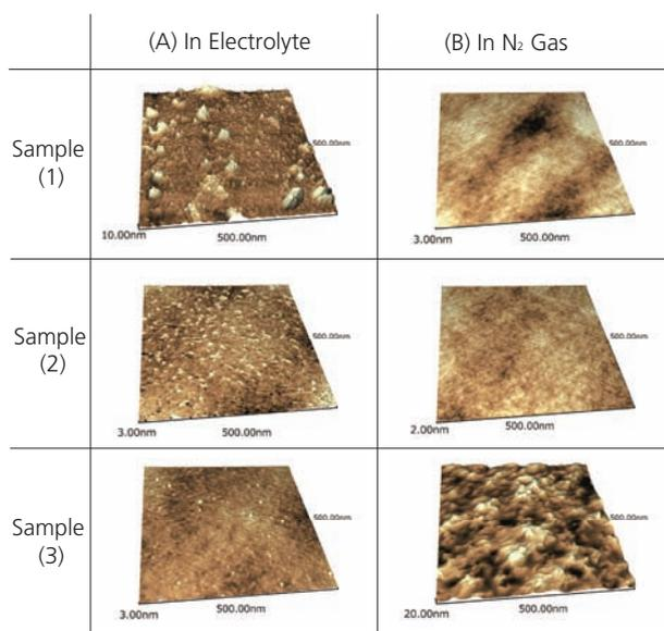
Fig. 5 Surface Morphology in Electrolyte and N<sub>2</sub> Gas (250,000 × magnification)
