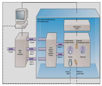
Figure 1. Schematic overview of the SMS DVS-Advantage instrument.
