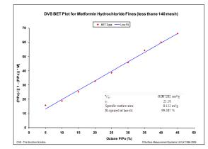
Figure 14. BET surface area plot for a hydrophobic drug using octane vapour at 25 °C.
