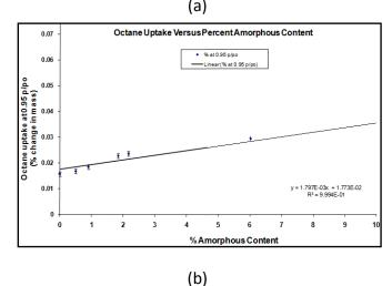
Figure 9. Octane vapor sorption isotherms (a.) and resulting calibration curve (b.) for lactose samples with various amorphous fractions.
