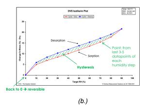
Figure 2. Moisture sorption kinetic (a.) and isotherm (b.) plots for starch at 25  $^{\circ}$ C.
