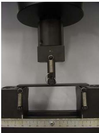
Fig. 2: Flexural Testing Status
