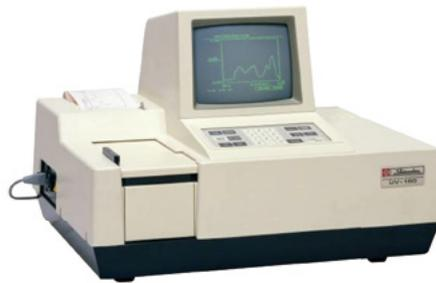
Fig. 7 Shimadzu UV-160 UV-VIS Spectrophotometer
