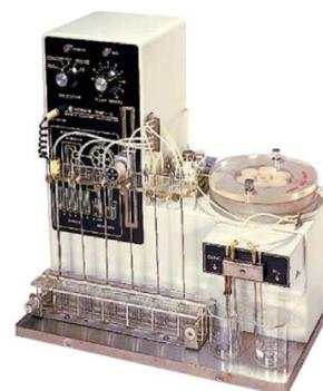
DGF-U Hitachi density gradient fractionator
