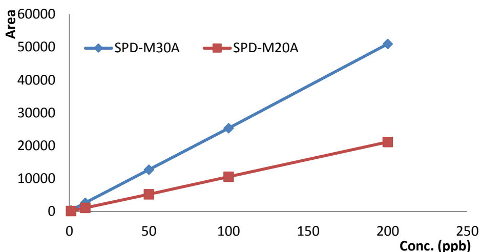
Fig 2: Calibration curves of anthracene std with SPD-M30A and SPD-M20A
